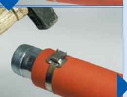
Hold stub of band with thumb, hammer it flat over bridge of buckle, complete clamp by hammering ears over stub.
