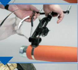
Pull on cutter lever, band is cut off to correct length.
