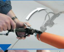
Place band in tool, push down on gripper with thumb, tension clamp by turning handle. Maximum tension is reached when band stops moving through buckle. When required tension has been applied, roll tool over buckle, at the same time reversing handle carefully approx. 1/2 turn to avoid breakage. There is no loss of tension, if handle is not reversed too much.
