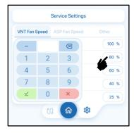
**Accessing VNT Fan Speed Settings:** In the Service Settings page, navigate to the VNT Fan Speed tab to modify the 5 preset fan speed values for the ventilator fan.
