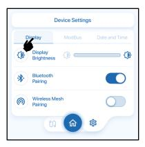
**Accessing Display Settings:** In the Device Settings page, navigate to the Display tab to modify settings related to your Touch Display.
