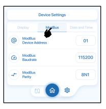
**Accessing Modbus Settings:** Navigate to the Device Settings page, and under the Modbus tab, customize various settings related to the Modbus connection.
